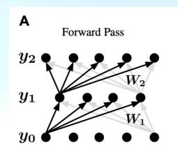
Output:  $y_l = f(h_l)$ Transfer Function: f(h)Activation:  $h_l = W_l y_{l-1}$  B Error Computation Loss Function: L  $\frac{\partial L}{\partial W_i} = \delta_i \times y_{i-1}$
